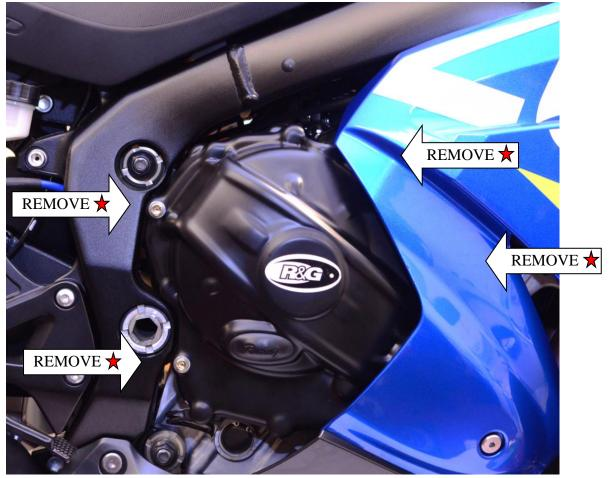
In this kit there should be: 1x Engine Case Cover (ECC0231R) 4x M6 x 40mm Long Cap Head Bolts 4x Spacers (S0820) 4x M6 Washers 1x Racing Puck (SK0001SK (already fitted)). 2x PAL Nuts (already fitted).
