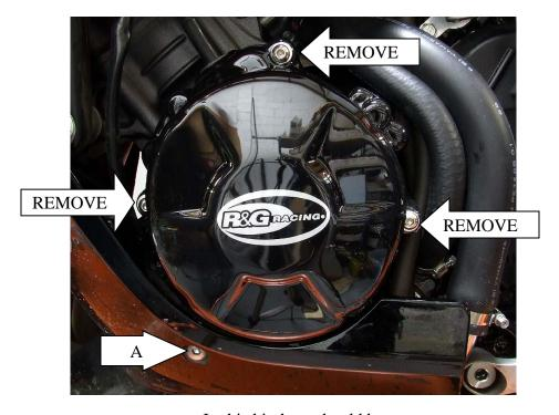
In this kit there should be 1 x Engine Case Cover (ECC0021) 3 x M6x40mm CAP HEAD BOLTS
